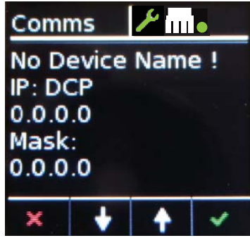
Figure 43 E-Pack 'Comms' screen display 'as-delivered' (Device Name = "", IP Configuration = Null).
